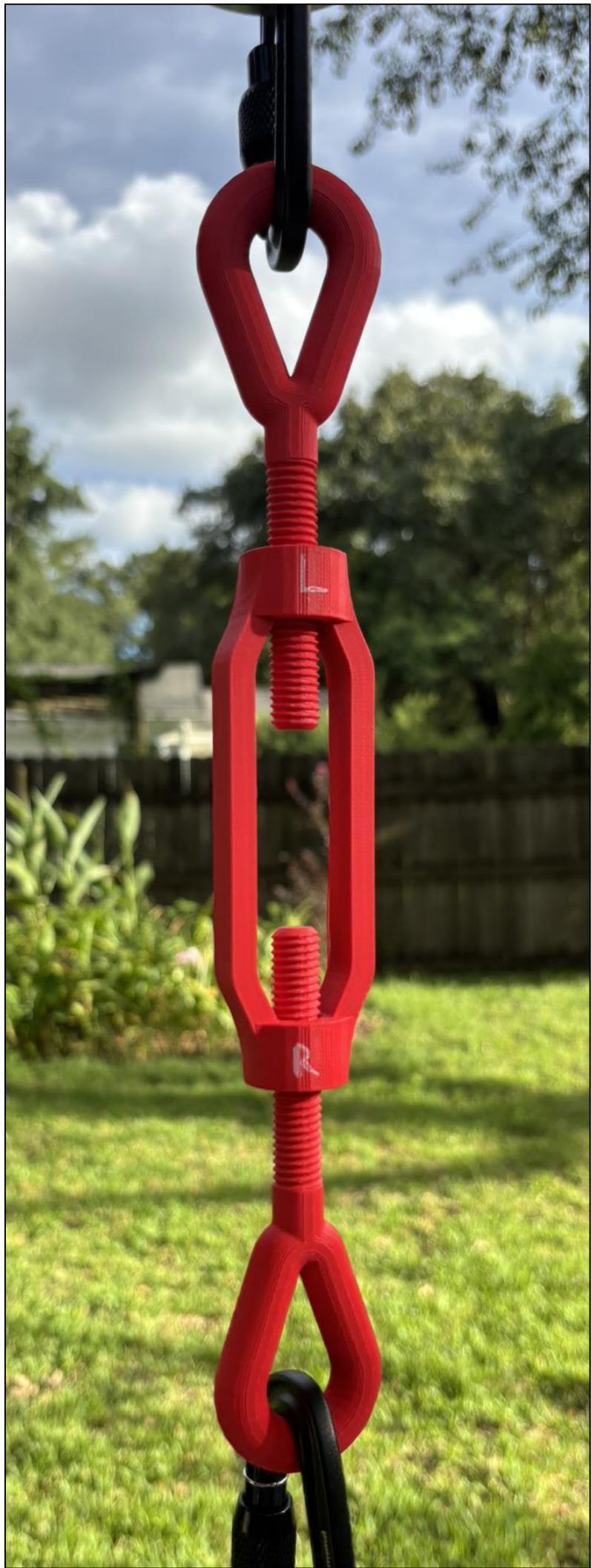
A 3D printed turnbuckle capable of holding 250lbs+.
