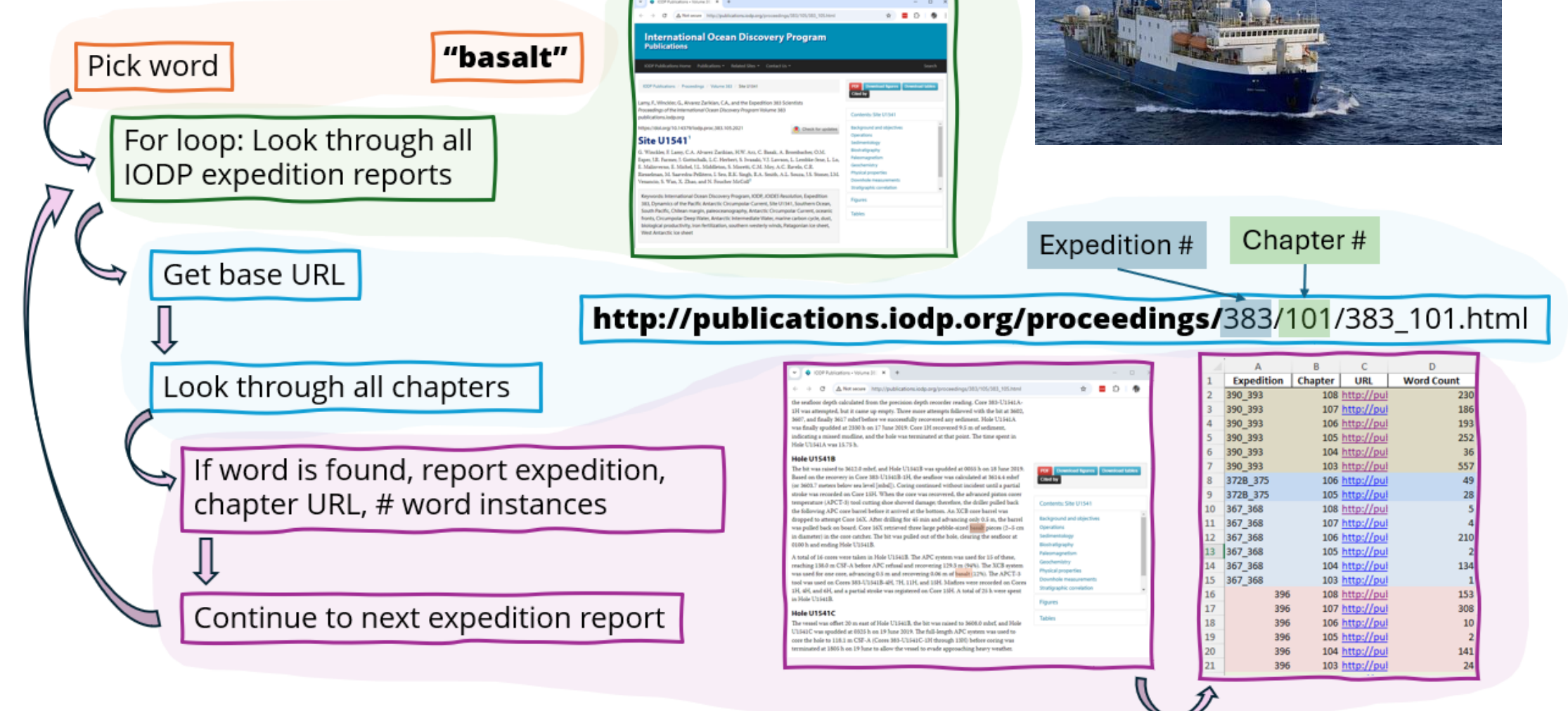
Figure 5 (above). Schematic representing the logic used to scrape the web for reports of contact with basalt while sediment coring.
