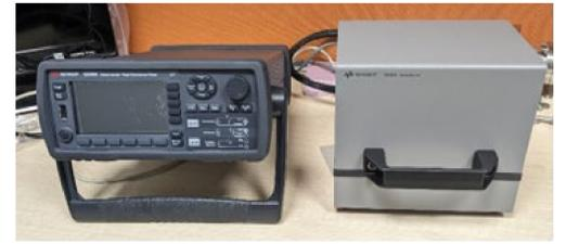
Keysight electrical conductivity measurement cell
